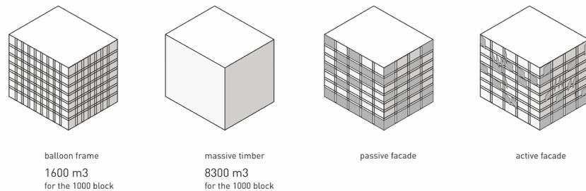
Features: The smaller the ratio between the perimeter of the building and its area, the higher the energy efficiency. Above the ground block increase the energy demand of 14% for heating and 50% for cooling in comparison with the partially underground solutions. It is necessary that the building is located end to the direction of the wind. The structural wood is much more economical and visually facilitates the construction of high-rise towers
