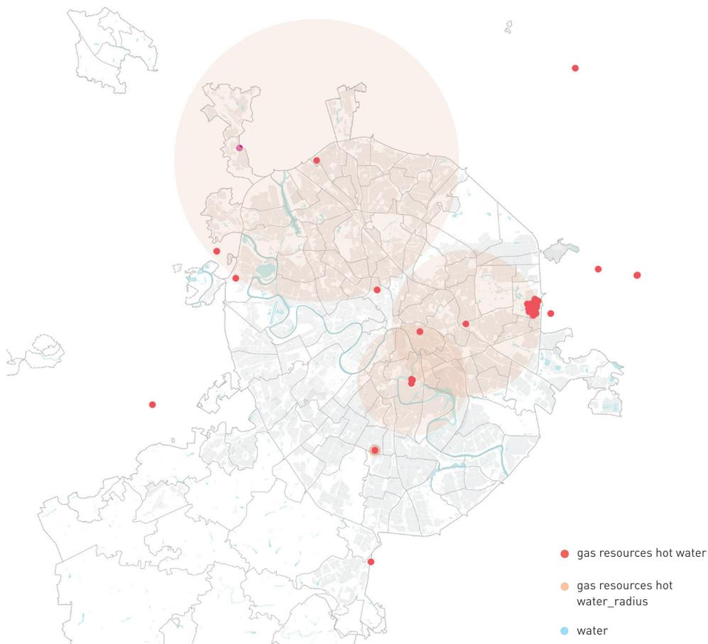
Water heating for the city is usually done using residue heat from the power stations or from Boiler stations located within the city. For power stations which produce the heat
